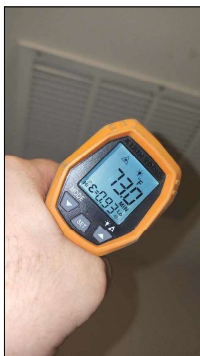
Differential temps at return look good. Should be 13 to 20 degree difference.
